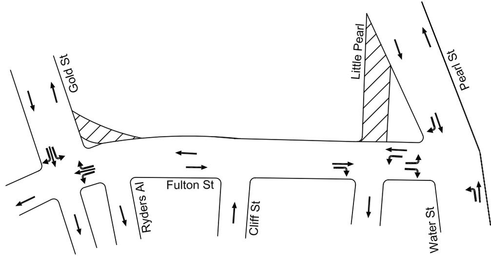
**PROPOSED GEOMETRY AND TURNING MOVEMENTS**
